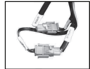
Connect Upper and Lower Cables
